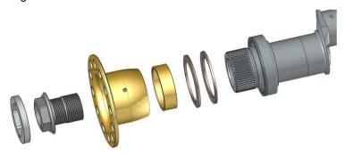
The propeller must be carefully selected to match the airframe and the engine characteristics. The hub of the propeller must be drilled with holes to match the flange. 6 propeller drive lugs are provided with the engine. These are made to have a tight fit in the propeller flange holes.
